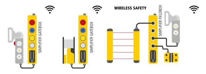
Indepedantly of CAN or wireless safety, all information reaches the Siemens controller via the Simplifier Gateway on PROFIsafe and can be programmed and managed centrally in the TIA programming software.
